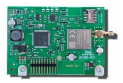
**ABS-LTE** is the new LTE communicator specifically designed for Absoluta Series control panels.
